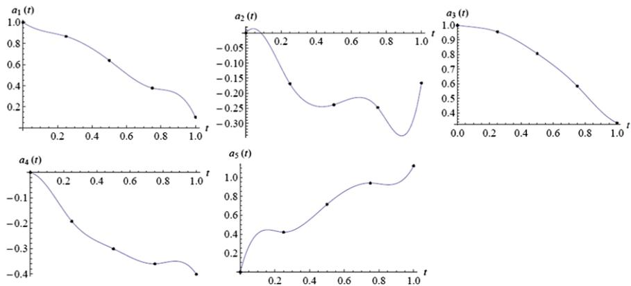
**Fig. 3** Kinematic B-spline solutions  $a_i(t)$  plotted versus time  $t \in [0, 1]$ , with  $F = 4$  sub-intervals
