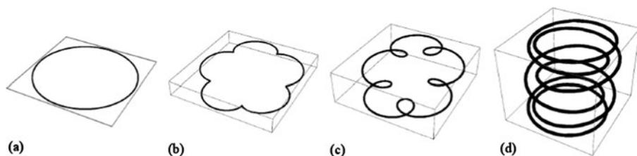
**Fig. 2** Five coil formations generated by (3) for  $n_1 = 1$  and  $n_2 = 6$  and kinematic parameters  $a_1(t) = a_3(t) = 1, a_2(t) = a_4(t) = -t,$  and  $a_5(t) = t.$  The initial circular configuration (a) writhes and folds in space in 5 different places (b)–(c) to produce 5 final coils (d)
