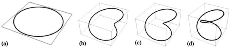
**Fig. 1** Single coil formation generated by (3) for  $n_1 = 1$  and  $n_2 = 2$  and kinematic parameters  $a_1(t) = a_3(t) = 1, a_2(t) = a_4(t) = -t$ , and  $a_5(t) = t$ . The initial circular configuration (a) writhes and folds in space (b)–(c) to produce the final coil (d)
